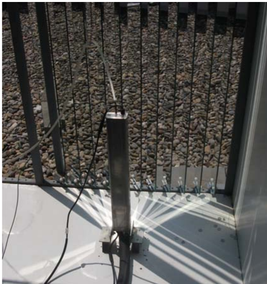
Figure 1.13 Example of Fresnel-transmission optical concentrator used in concentrating photovoltaics systems.
