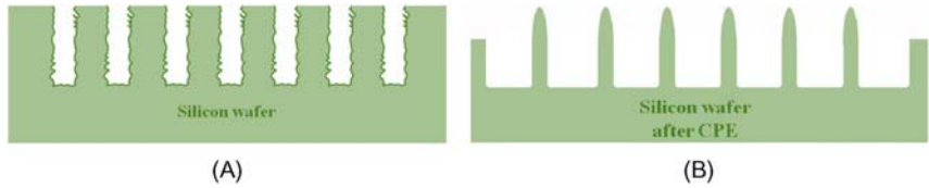
Figure 9.9 (A) Schematic diagram of the fabrication of silicon nanoholes with surface defects and metal contamination. (B) Schematic diagram of silicon nanostructures after CPE treatment. CPE , Chemical polishing etching.
